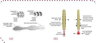
Figure 1. Anchorage behavior of the bio-analogs: (a) earthworm muscle expansion and contraction and extension of bristles into the soil for anchorage, (b) razor clam bi-valve shell expansion and contraction for anchorage
